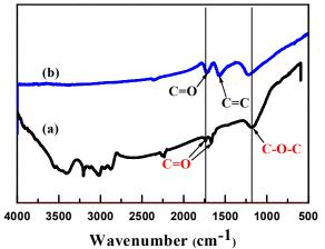
Fig. 4: FTIR spectra of the CNT (a) and the as-prepared GNS (b).
