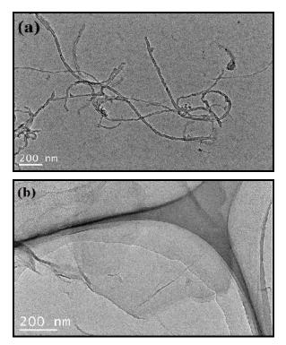
Fig. 2: TEM images of the CNT (a) and the as-prepared GNS (b).
