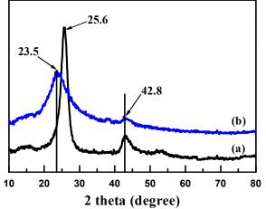
Fig. 3: XRD spectra of the CNT (a) and the as-prepared GNS (b).
