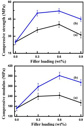
Fig. 6: Compressive strength and modulus of the PF/CNT (a) and PF/GNS (b) composites.
