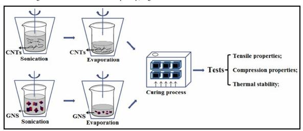
Fig. 1: Fabrication and characterization of the PF/CNT and PF/GNS composites.
