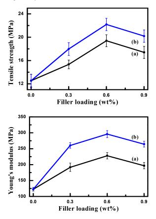
Fig. 5: Tensile strength and Young's modulus of the PF/CNT (a) PF/GNS (b) composites.
