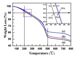
Fig. 7 TGA spectra of the pure PF (a), PF/CNT (b) and PF/GNS (c) composites (The filler loading was 0.6wt%).
