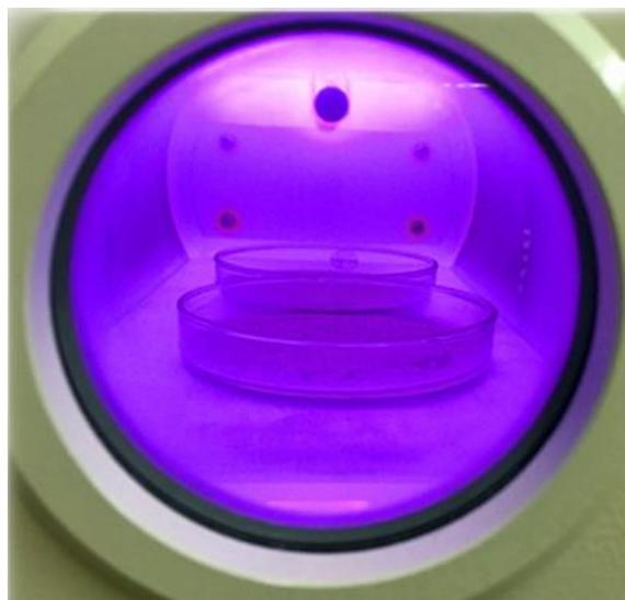
Fig. 1: b. Image of the glow discharge process.
