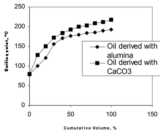
Fig. 1: ASTM distillation curves of oils derived from catalytic pyrolysis of waste rubber tube at 350 °C.
