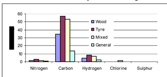
Fig. 2: Ultimate analysis results of auto shredder waste streams and wood.
